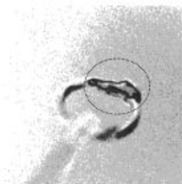
Fig. 7 Thermograph of a Phoenician ring. In the circled area, the volume of material used to weld the collet to the ring support can be easily observed, even though partly hidden under the outer gold leaf coating
