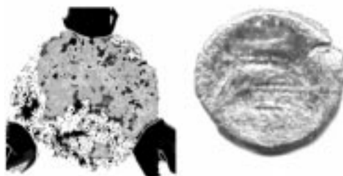
Fig. 8 Thermograph of a Roman coin (left side). Two main different areas reveal an inhomogeneity in the material composition. On the right side the corresponding photograph from which no evidence of such inhomogeneity can be detected
